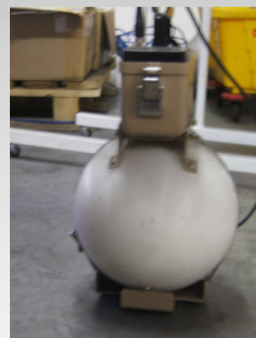
Radiation survey meter. This is used when survey the area where the analyser is installed and the readings are recorded and analysed.
